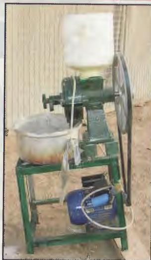
Grinder - used to crush AN and CAN
